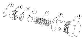
23-063 VLV, CHECK, CHECK VLV MANIFOLD
