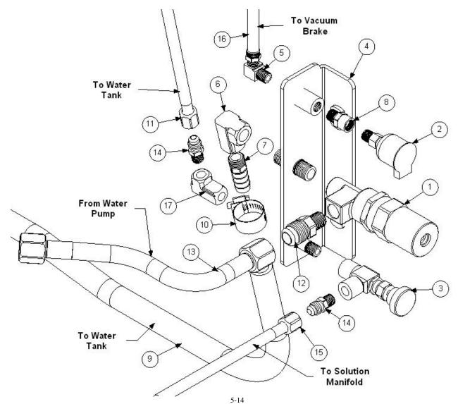
69-187 ASSEMBLY, BRACKET, MOUNTING, LOWER RIGHT
