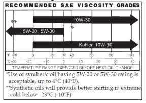
**NOTE:** Using a lower service class oil or extending oil change intervals longer than recommended can cause engine damage.
